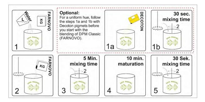
**Processing:** DPM Classic can be applied by brush, roller and airless spraying(nozzle 0,025" – 0,031"; spray pressure 150 - 200bar; 5kg dissolved with ca.4l water). When preparing the material, follow the instruction steps below.
